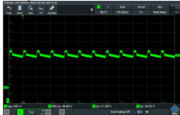
Oscillogram 2; 48 Vdc at 100 Hz
