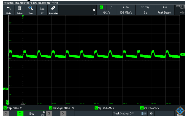
Oscillogram 4; 48 Vdc at 100 Hz
