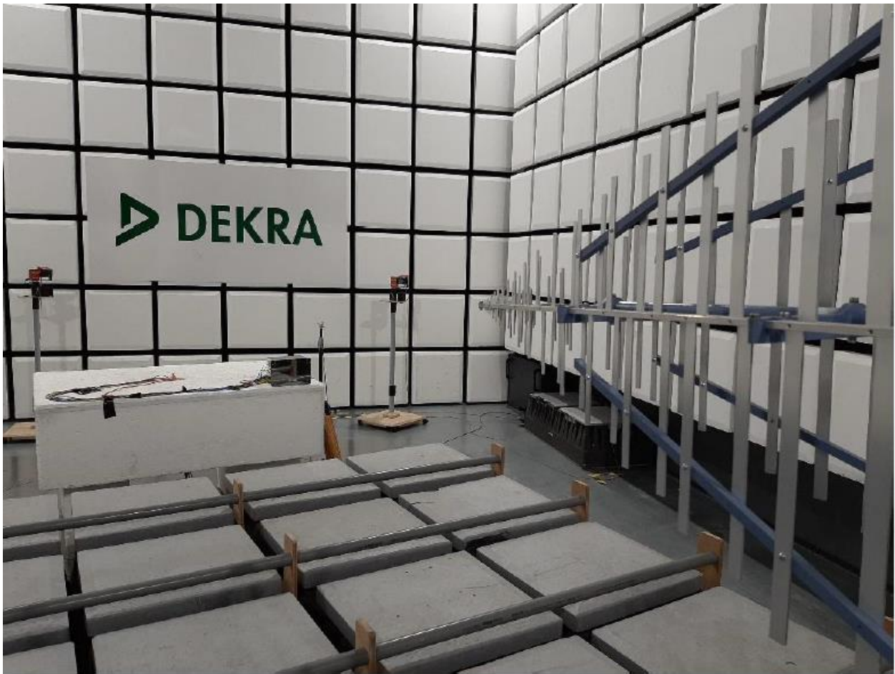
Radiated interference test setup, front side
