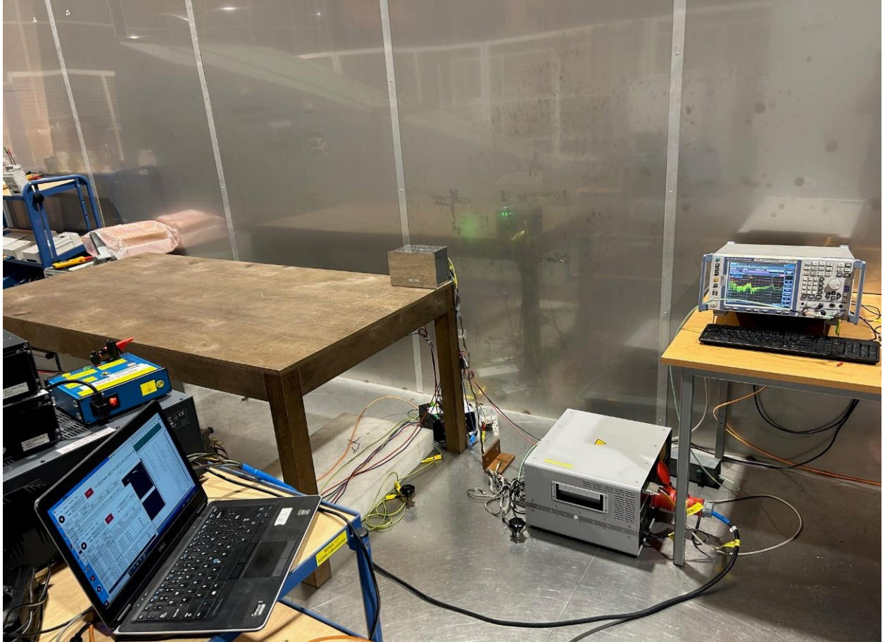
Conducted emission test setup
