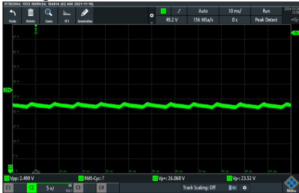
Oscillogram 1; 24 Vdc at 100 Hz
