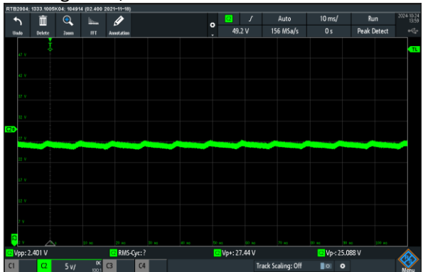
Oscillogram 3; 24 Vdc at 100 Hz
