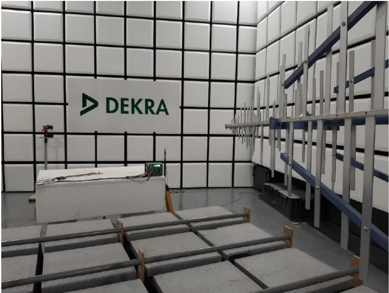
Radiated interference test setup, back side
