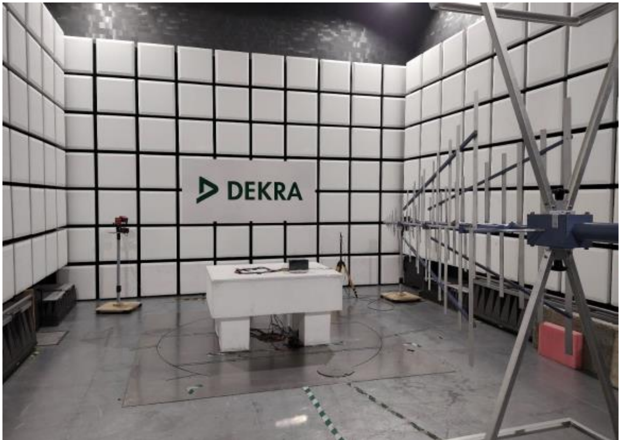
Radiated electromagnetic disturbances (30 – 1000 MHz)
