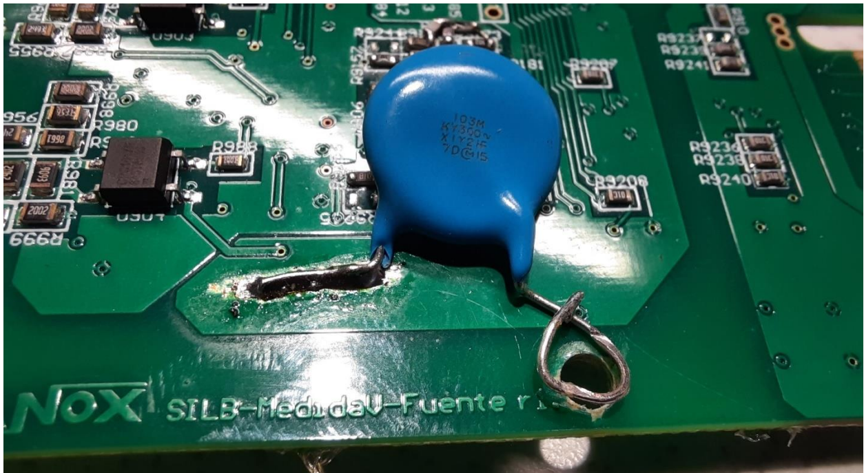
Surge arrester on SILB-MedidaV-Fuente board
