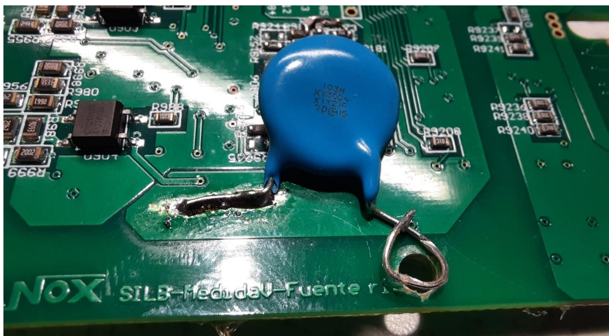
Surge arrester on SILB-MedidaV-Fuente board
