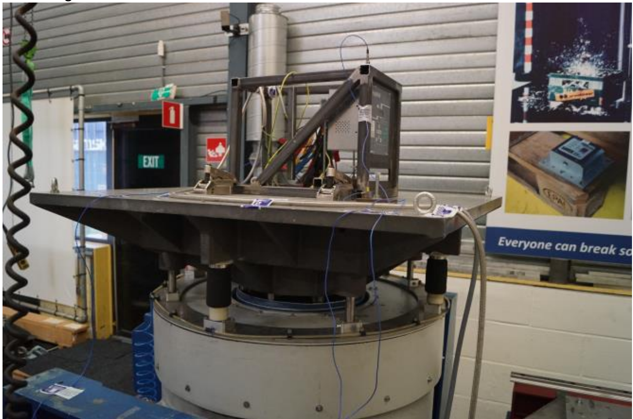
Test arrangement Z vertical direction
